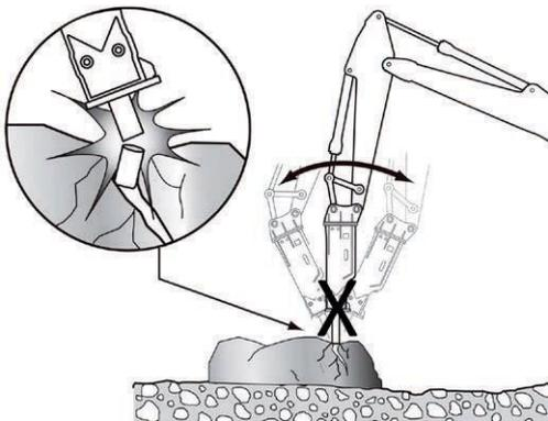
**Never strike the same spot for more than 30 seconds.** If rocks are especially hard avoid continually striking the same spot for more than 30 seconds. It is better practice to change target periodically which avoids raising the oil temperature. This can result in damage to the accumulator and excessive tool wear.
