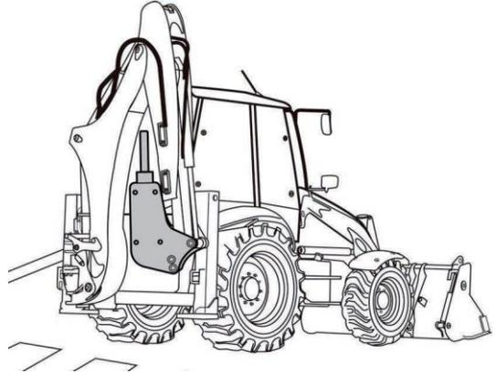
Backhoe Loader with breaker in travelling position
