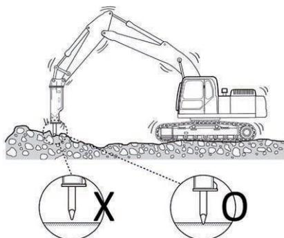
Conversely, if thrust is excessive or breaking is performed with boom of the carrier raised as shown below, the machine may suddenly tip toward the movement. The breaker body may strike the broken rocks violently resulting in damage.
