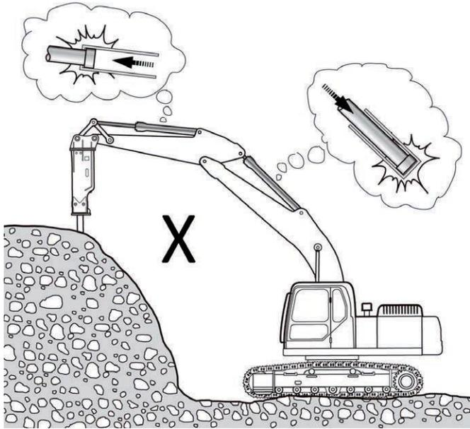
**Always warm the carrier up in cold conditions.** If the breaker is operating with low oil temperature the piston & seals are prone to damage. Warm the carrier up for five to twenty minutes. During this time operate the hydraulics to move the boom. Oil temperature must reach min. 0°C before operating the breaker. (Please refer to Carrier Operator's Manual).
