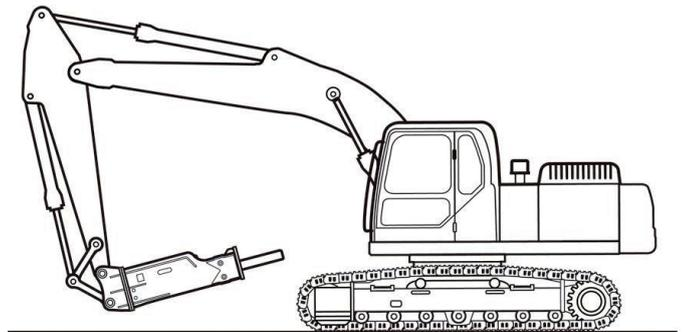
Excavator / Compact excavator with breaker in travelling position
