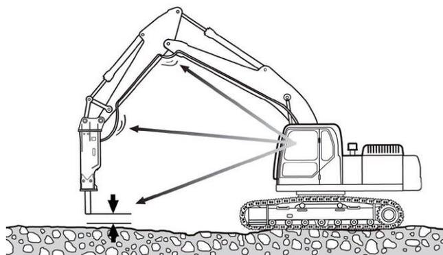
**Stop as soon as breaking is completed.** As soon as rocks are broken, cease power to the breaker. If idle striking continues the accumulator may be damaged, the bolts loosened or broken and also damage may be caused to the excavator. When a proper thrust is not applied to the breaker or the tool is used as a lever, the state of idle striking will occur. (Idle striking makes a higher pitched ringing sound).
