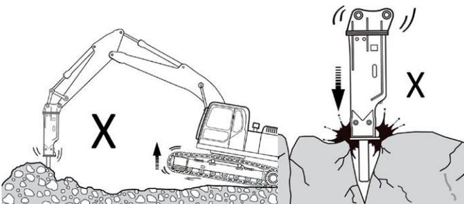
Excessive force as above may also result in vibrations being transmitted to the tracks causing damage.
