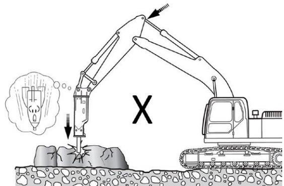
**Never strike with the cylinders of carrier extended to the end of stroke.** Excavator cylinder damage may be caused if the breaker is operated with the arm fully extended.
