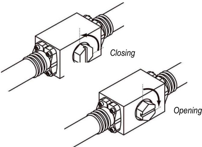
Opening and closing of the stop valve (Split type)
