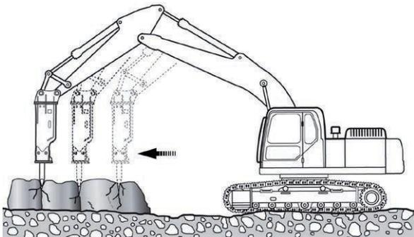
**On a hard, large rock, start breaking at the end point. (advance).** Begin with a target near the end of a large
