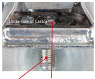
Castor mounting bolt Swivel bearing head should feel free to rotate and not loose
