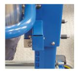
Pic 1. Mast interlock with cover on
