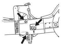
Dismantle the old blades by loosening the centre nut. Check the drive belt for wear when the blades are dismantled. When changing the drive belt see the instructions under the heading "Replacing the drive belt".
